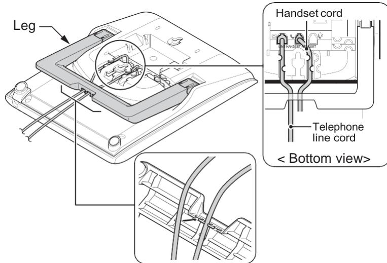
**Figure 2-91 Cabling for Wall-Mount**
