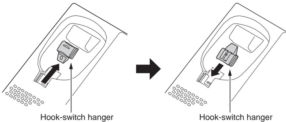
**Figure 2-92 Hook-Switch Hanger**
