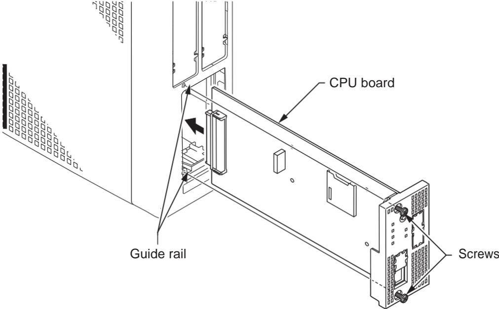
**Figure 4-7 Installing the CPU Board**
