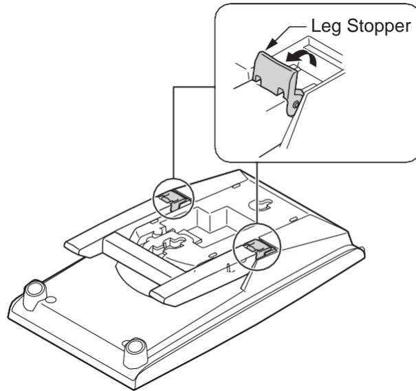
**Figure 2-105 Leg Stopper of DSS Console**
