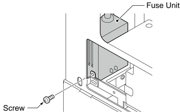
**Figure 2-51 Loosen the Fuse Unit Screw**
