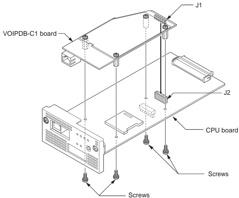
**Figure 2-79 Installing the VOIPDB-C1 Board**
