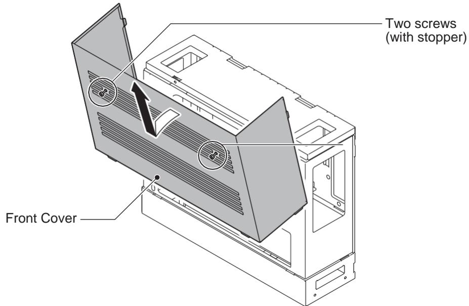
**Figure 2-27 Removing the Front Cover**
