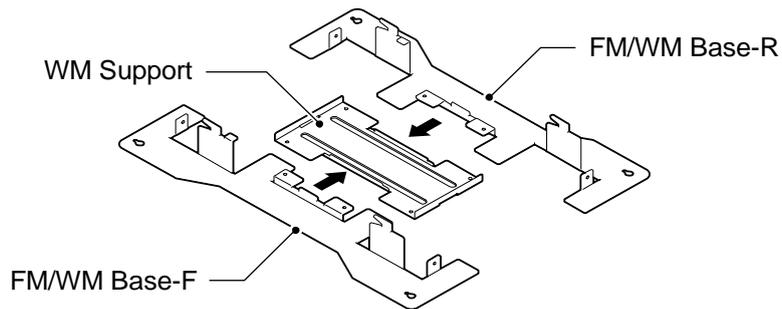
**Figure 2-39 Bases and Support of the Battery Box**
