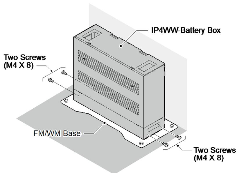
**Figure 2-42 Securing the Battery Box**
