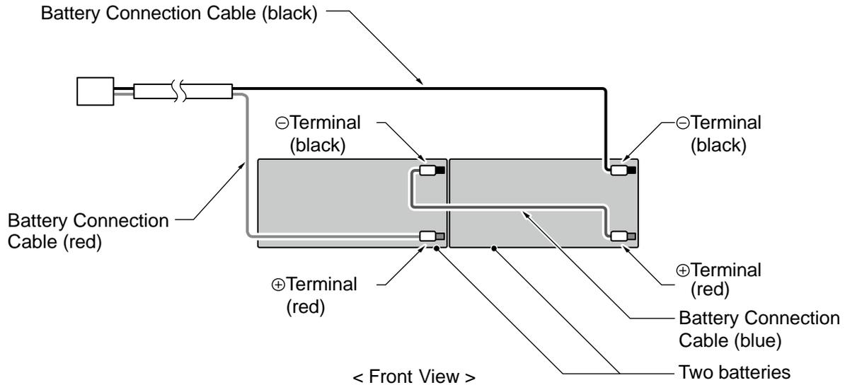
**Figure 2-33 Connecting the Battery Cables**
