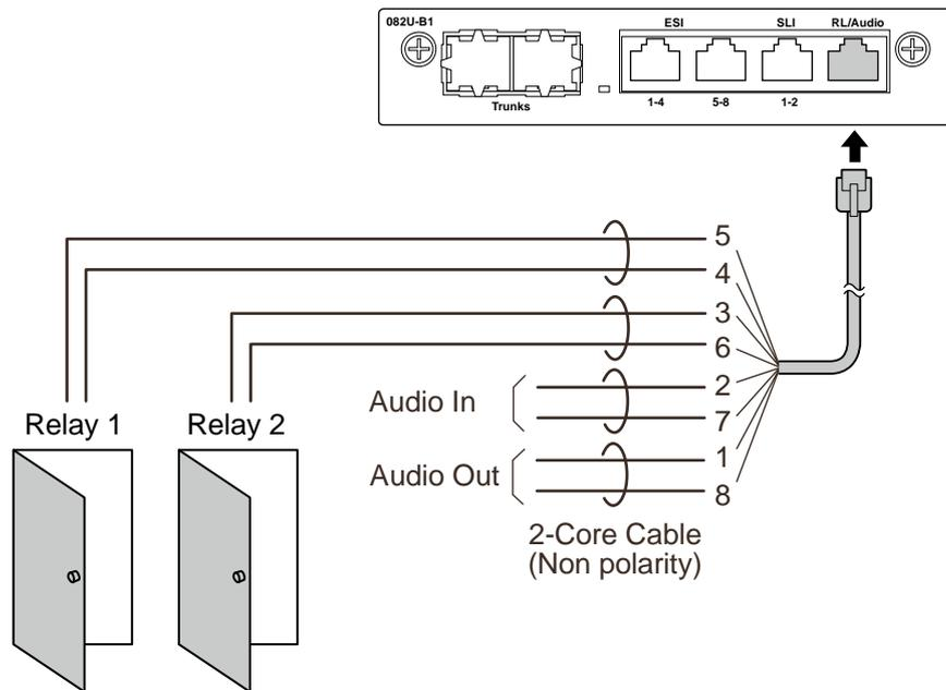
**Figure 2-120 Connecting the Door Unlock Device (082U-B1)**
