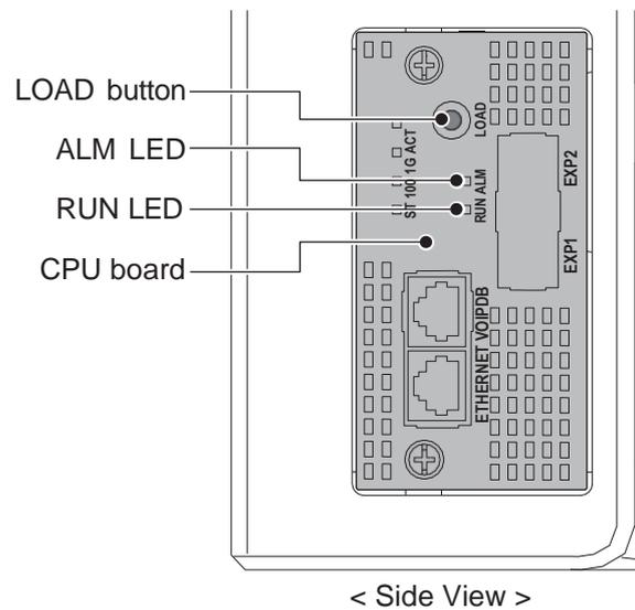
**Figure 3-2 ALM LED and RUN LED Location**
