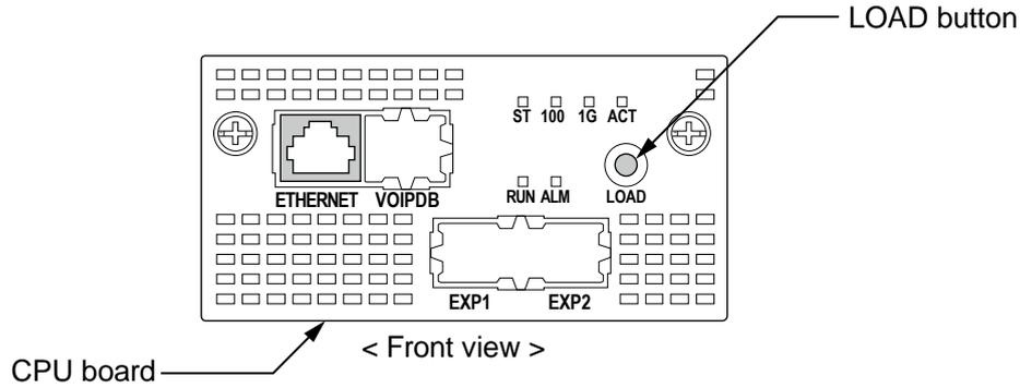
**Figure 4-11 Push in and hold the LOAD button**
