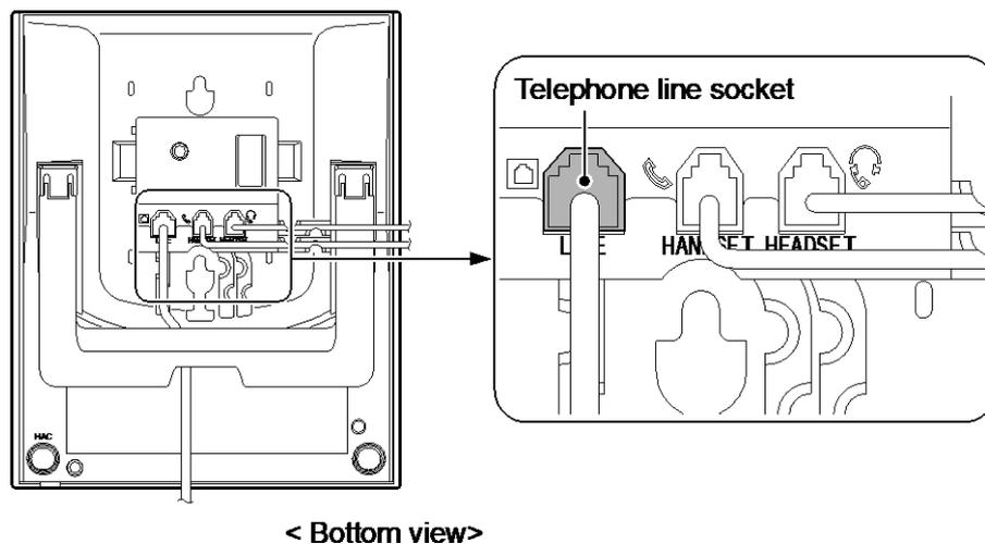
**Figure 2-126 Telephone Line Socket (Digital Multiline Telephone)**
