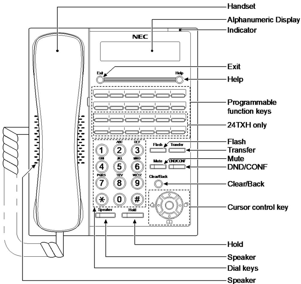
Figure 2-85 Hybrid Multiline Telephone (12TXH-A1/24TXH-A1)
