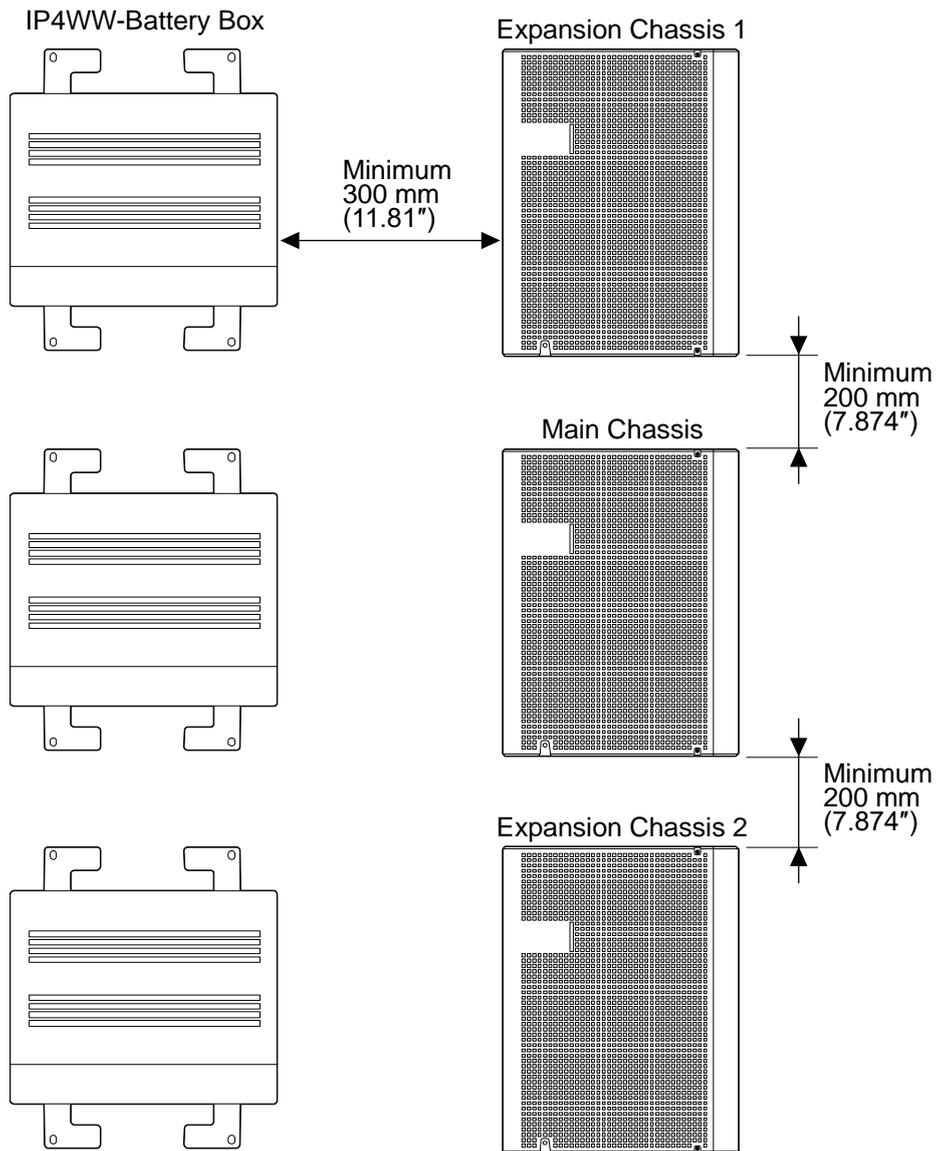
**Figure 2-13 Vertical Arrangement of Chassis and Battery Boxes**
