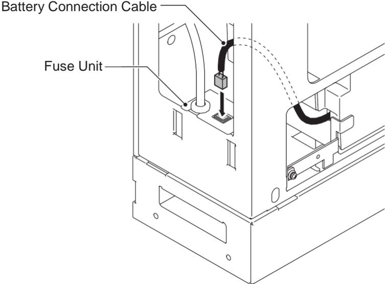
**Figure 2-55 Connect Battery Connection Cable**
