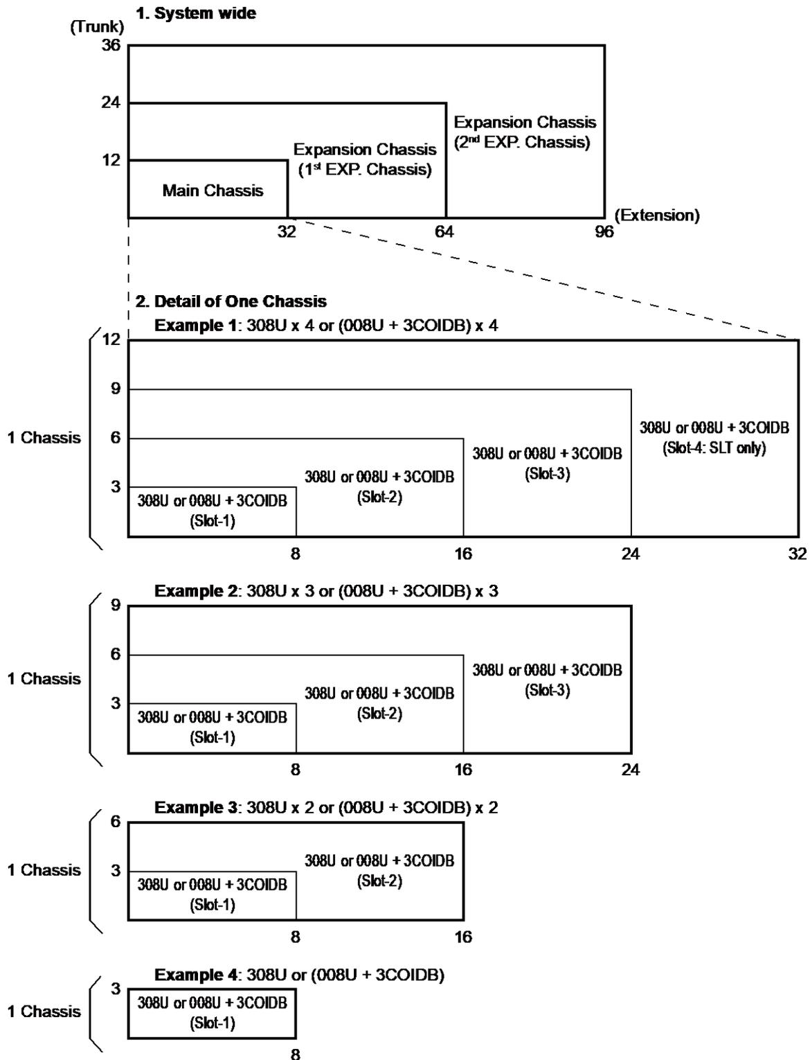
Figure 1-3 Expandability of Trunk and Extension (without BRI/PRT)
