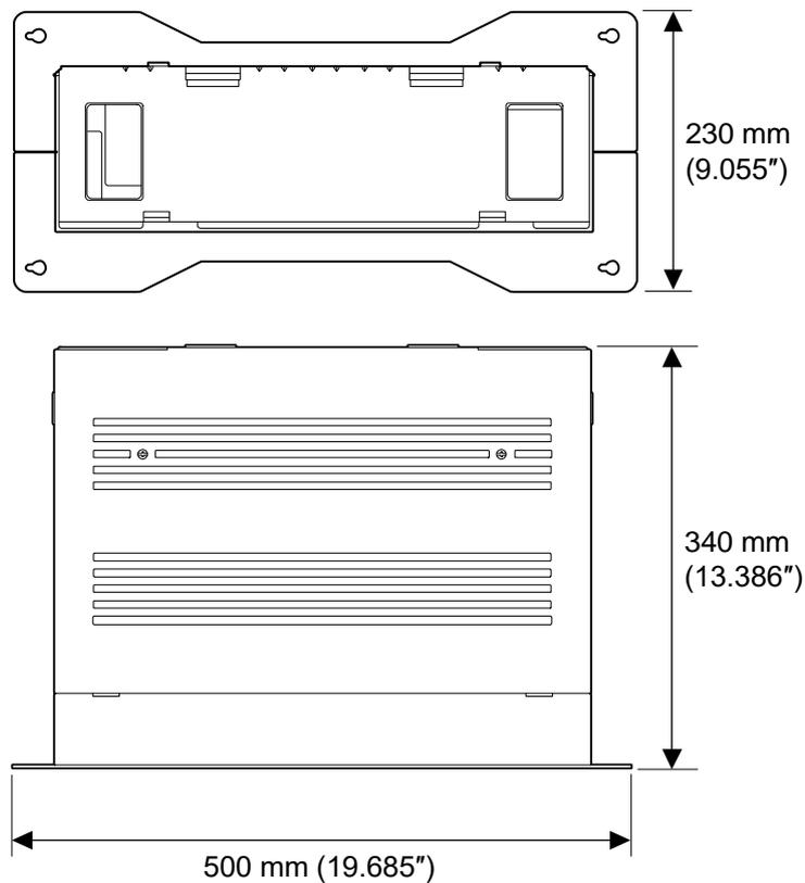
**Figure 2-26 Dimension of the IP4WW-Battery Box**
