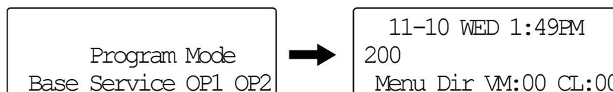
**Figure 3-12 Exiting Programming Mode Display 2 (12TXH/24TXH-B1)**
