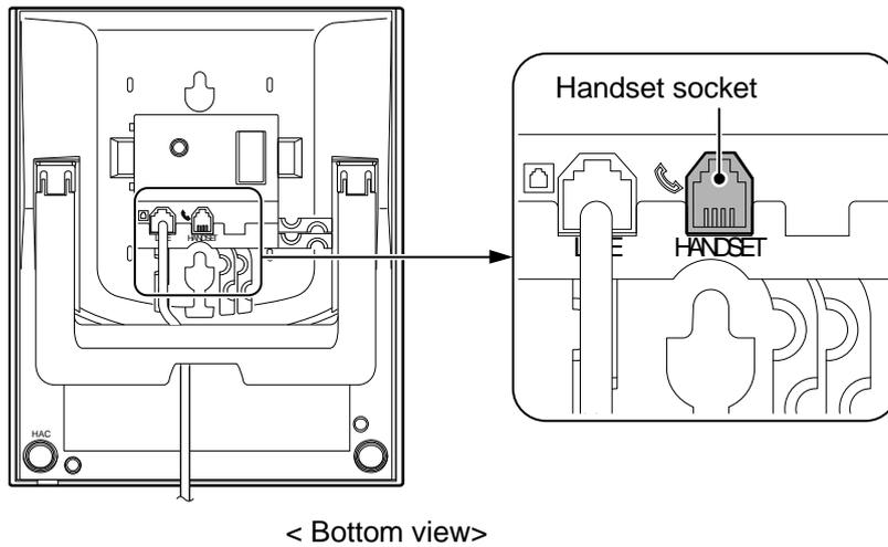
**Figure 2-110 Headset Socket (4W Hybrid Multiline Telephone)**
