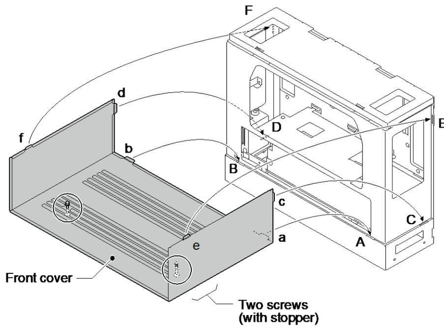
**Figure 2-56 Installation of the Front Cover**
