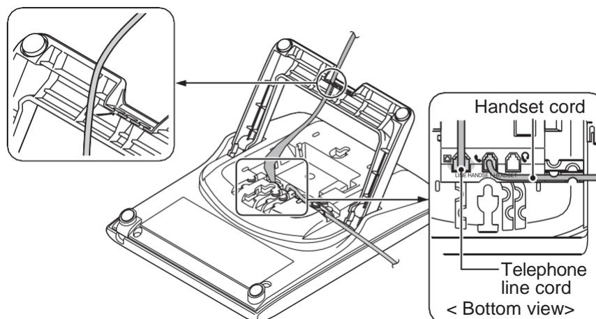
**Figure 2-88 Cabling of Multiline Telephone**
