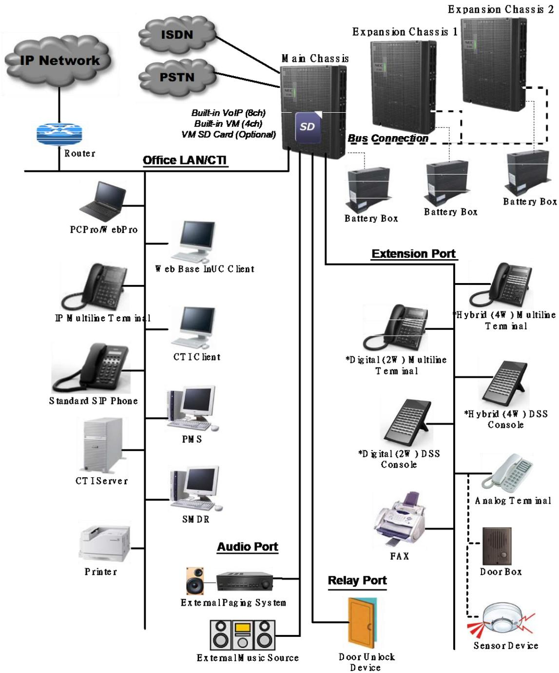
Figure 1-1 System Configuration
