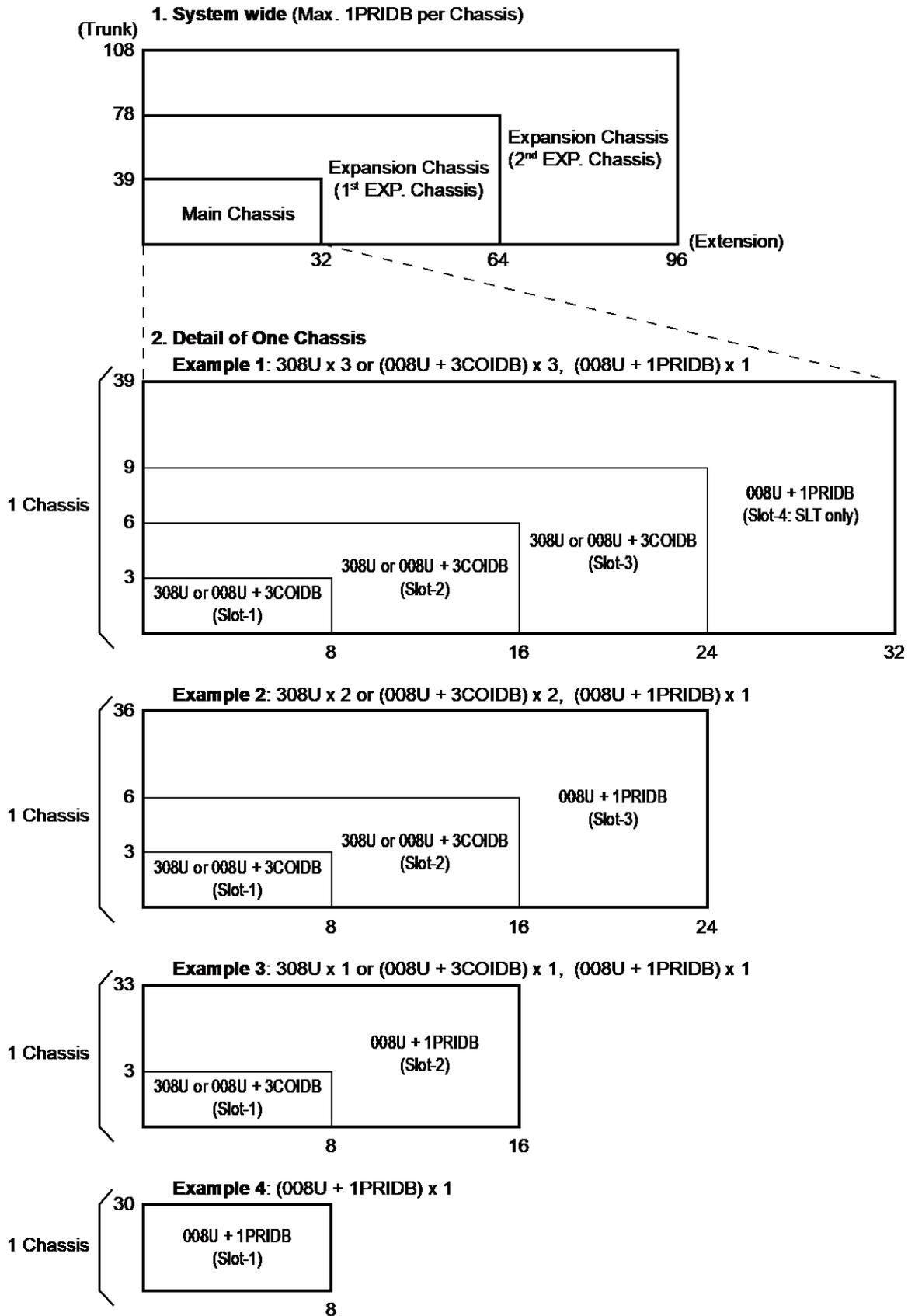
Figure 1-6 Expandability of Trunk and Extension (with PRI)
