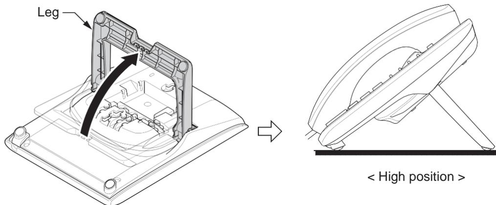
**Figure 2-90 Leg Setting for High Position**
