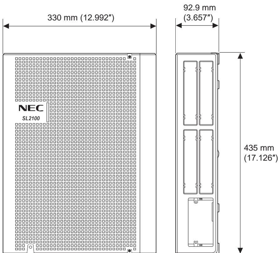
**Figure 2-6 Dimension of the Chassis**
