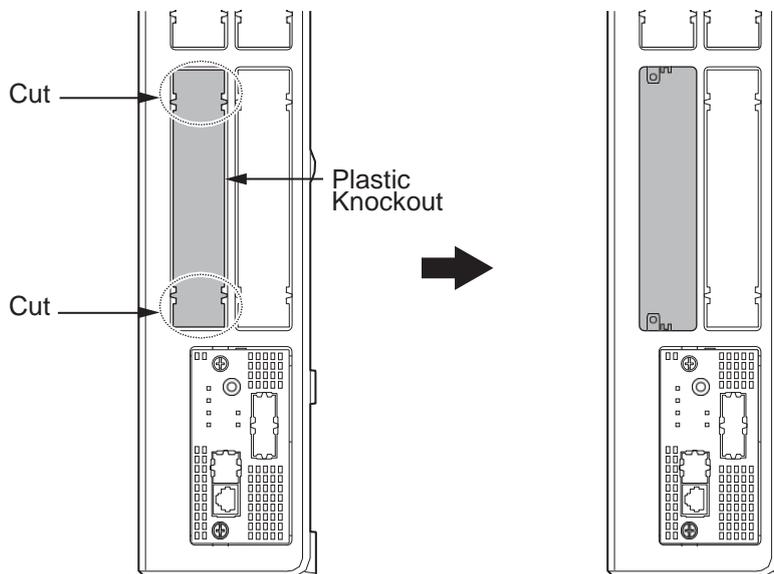
**Figure 2-58 Plastic Knockouts**
