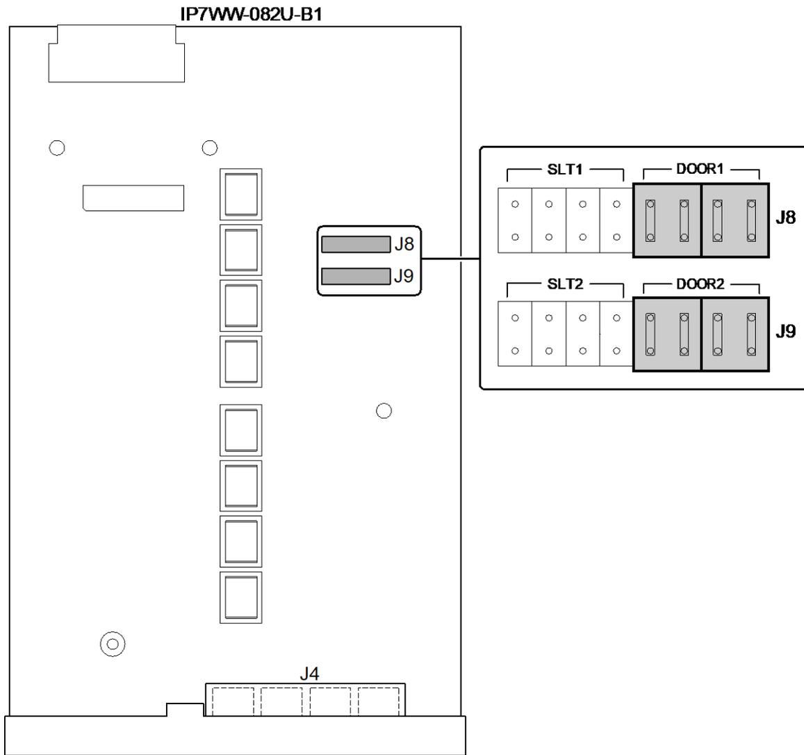
Figure 2-116 Switches Location of 082U-B1
