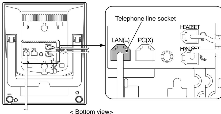
**Figure 2-127 Telephone Line Socket (IP Multiline Telephone)**
