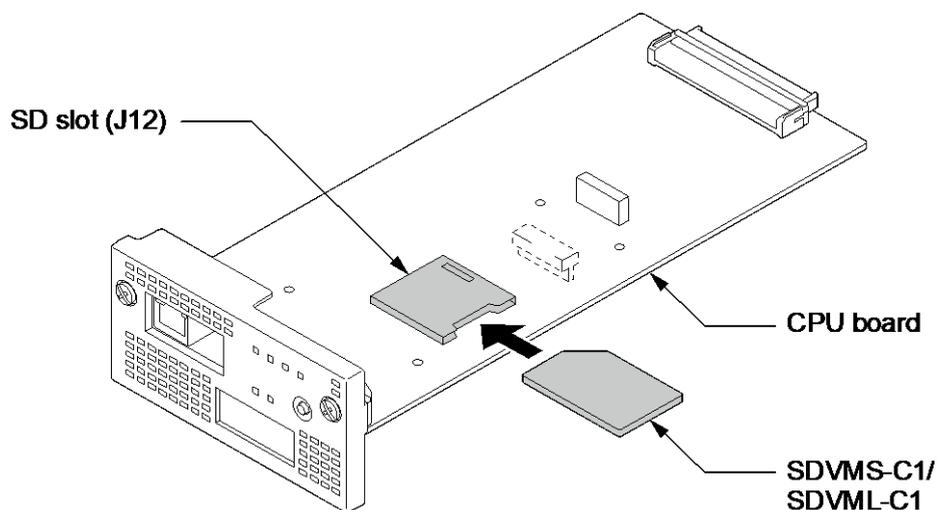
**Figure 2-84 Installing the SD Card**
