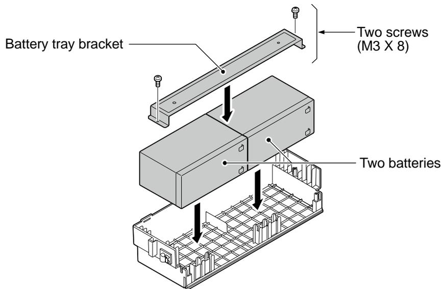
**Figure 2-32 Battery Installation**
