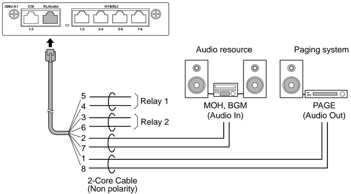
**Figure 2-121 Connecting Audio Equipment (308U-A1)**
