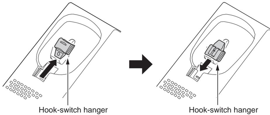
**Figure 2-100 Hook-Switch Hanger**
