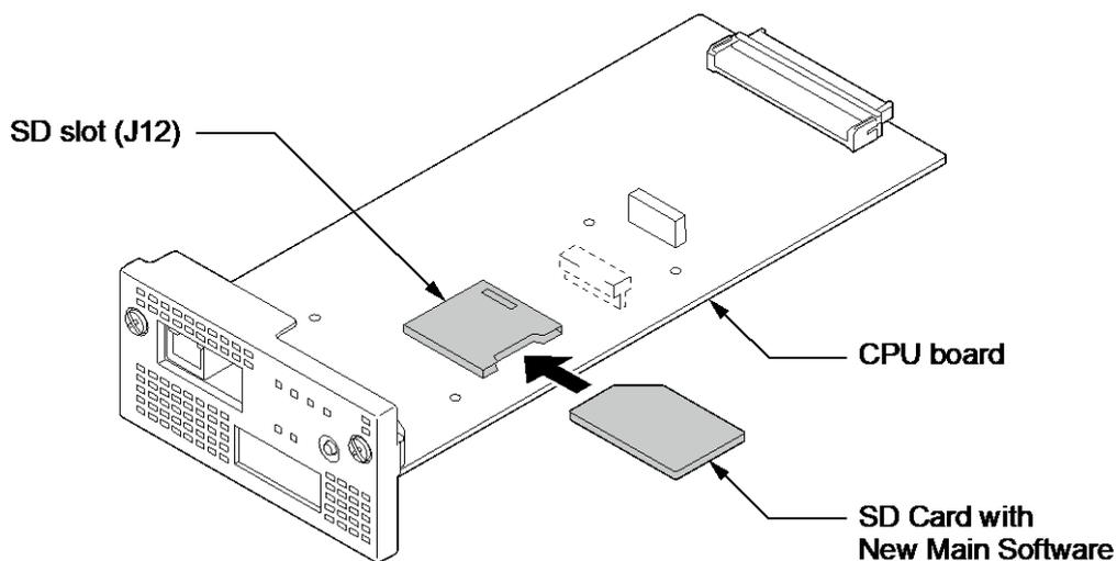
**Figure 4-10 Insert the SD card**
