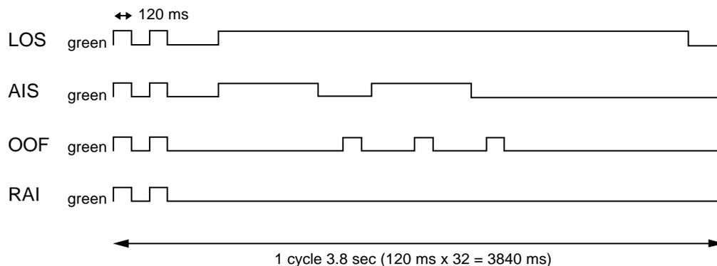
**Figure 2-75 Indication Pattern of Layer 1 on T1 Board**
