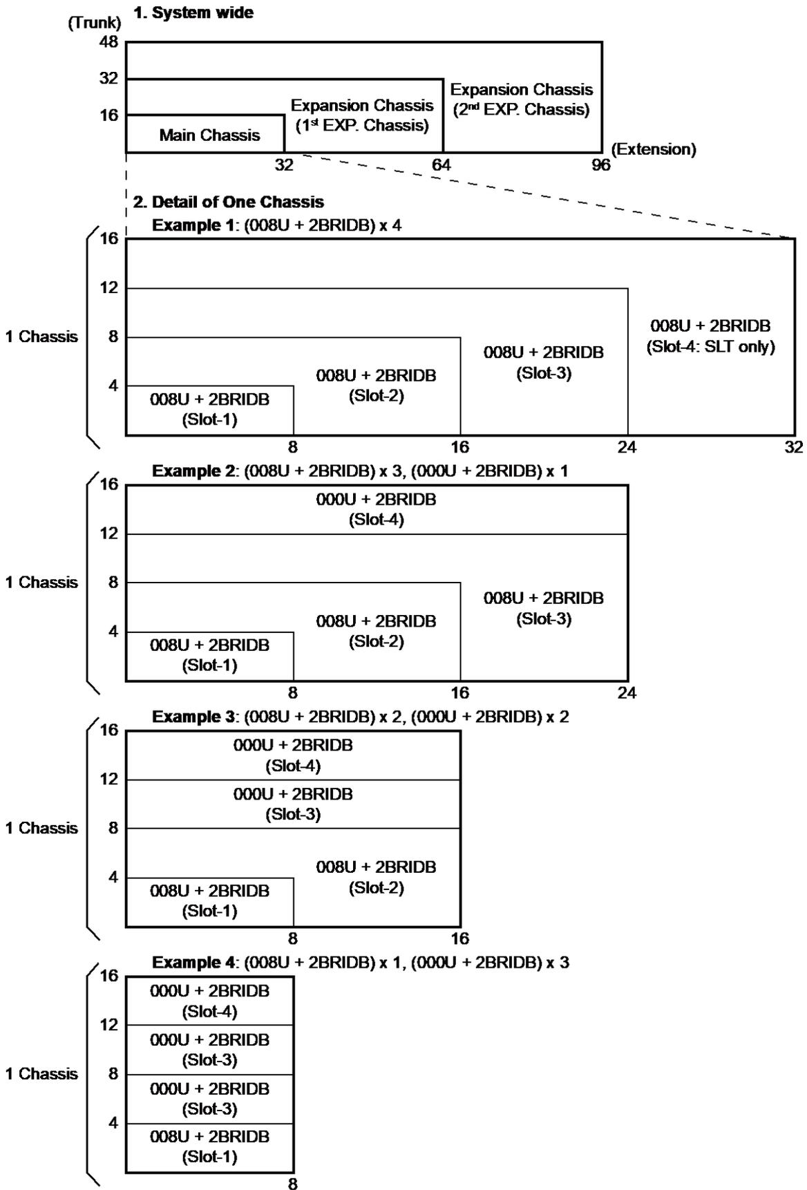
Figure 1-5 Expandability of Trunk and Extension (with BRI)
