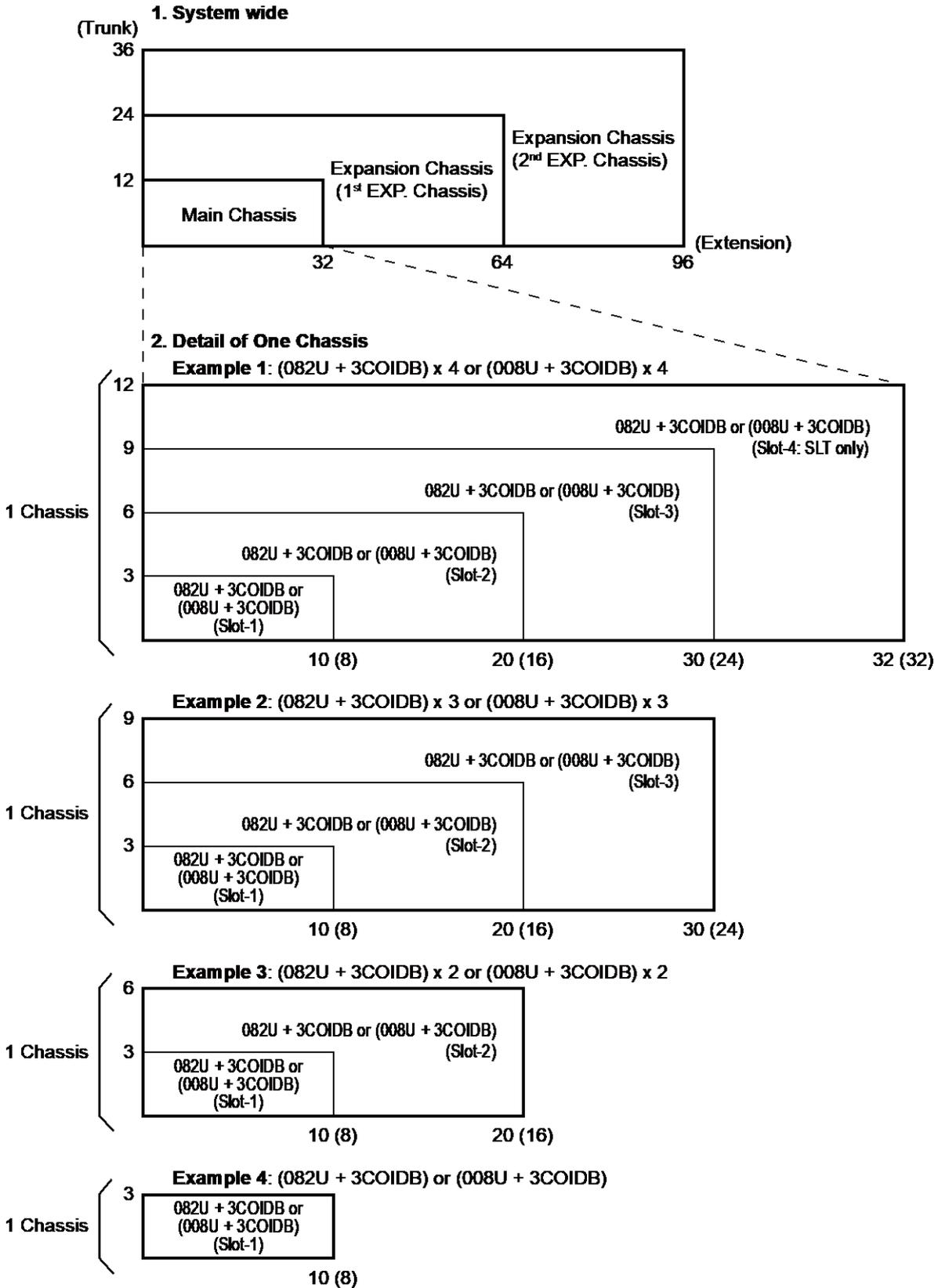
Figure 1-4 Expandability of Trunk and Extension (without BRI/PRT)
