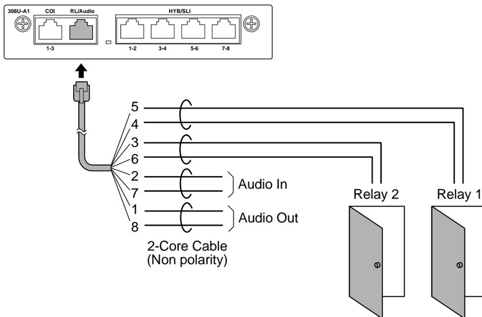
**Figure 2-119 Connecting the Door Unlock Device (308U-A1)**
