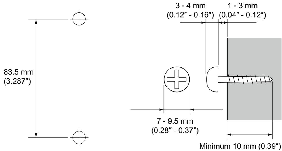
**Figure 2-93 Wall-Mount Screw Guide**
